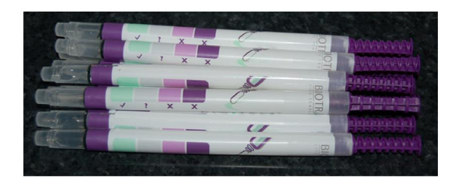
The liquid in the left side of the Pro-tect swabs changes colour from green to purple dependent on the concentration of protein residue on an environmental surface
