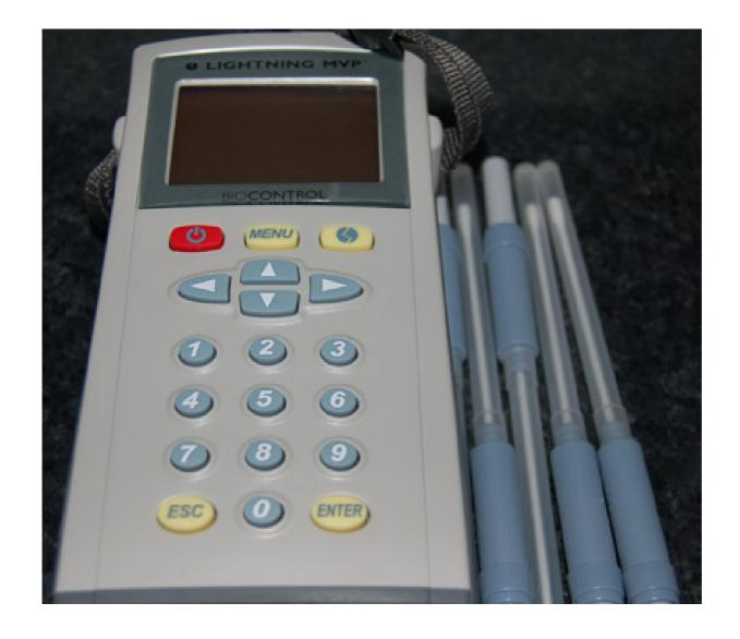
ATP detection involves the the use of a luminometer to measure how much light is produced from the contamination present on an environmental surface
