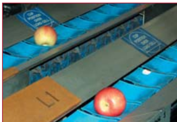
Photo 4. Sites on the packing line such as cups, that are in direct contact with fruit, should be kept clean
