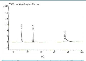
Figure 2. Chromatogram showing degradation of Vitavax by clover rhizobial strain TA1. HPLC-UV chromatograms analysis using C18 column. (a)-(e) show the degradation after 48, 96, 144, 196 and 240 hours of incubation.
