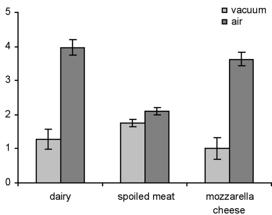
FIG. 4. Mean odor intensities ( \pm standard errors) of samples stored in air and in vacuum packs. Both the means and the standard errors were calculated across all the samples ( n = 10 ).
