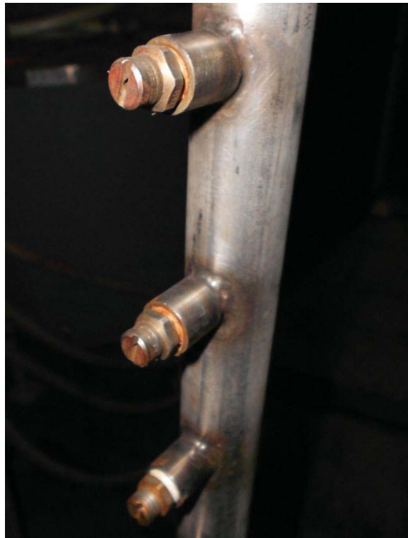
Figure 6.1 Commercially available spray wash nozzles attached to a rotating wand.
