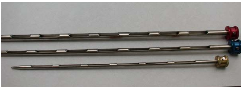
The illustration shows 3 different sizes of double sleeve triers.
