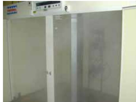
Figure 3. Electrostatic spraying of sanitizer in a hatching cabinet.
