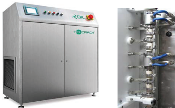
Fig. 1. 30 kW PEF system (left), treatment chamber setup (right)
