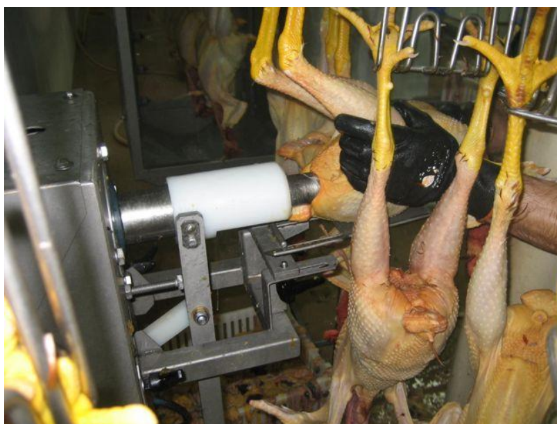
Figure 19. Bayle Annular Knife Vent Cutter machine with central vacuum
