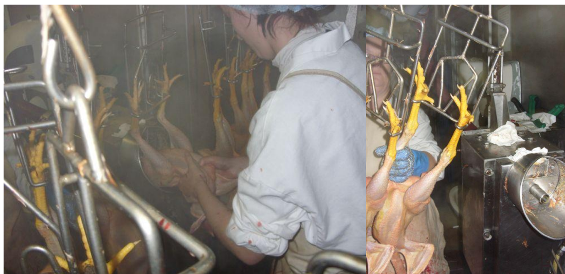
Figure 16. Machine based removal of intestine and duodenum (Plant B)
