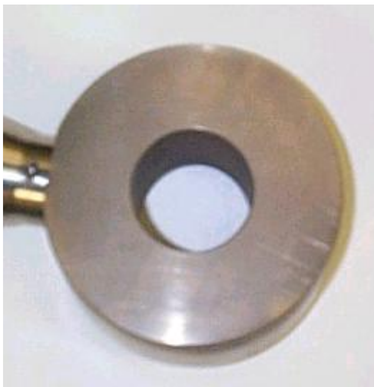
Figure 4. Photograph of an ultrasound radial cell applicator (20 kHz).
