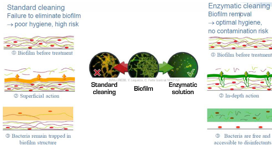
Fig. 1. Comparison of effectiveness between the traditional CIP and enzyme cleaning technique.
