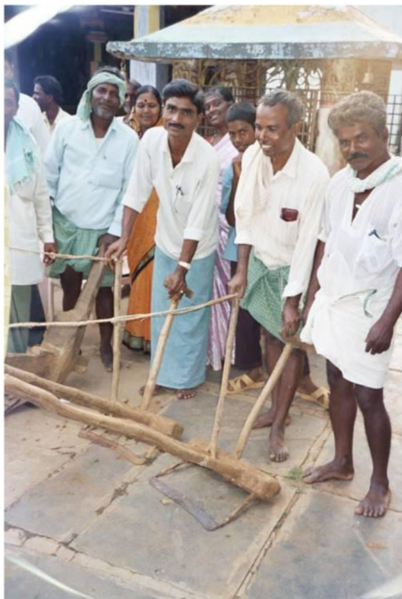
Figure 1 Demonstration of the yedekunte implement used by farmers in Karnataka state of India. The implement cuts weed roots below the soil surface between rows, thereby also aerating the top layer of soil (Norman Uphoff).
