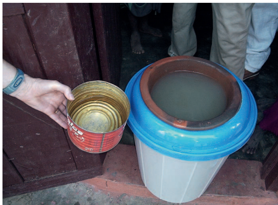
Fig 2 | The Kosim system. This consists of a ceramic pot filter that removes soil debris and microbiological contaminants from the water. The appearance of water from an earthen basin located in the Gonja District (Northern Ghana) is shown before (right) and after (left) the Kosim sanitation step. Picture courtesy of S. Murcott.
