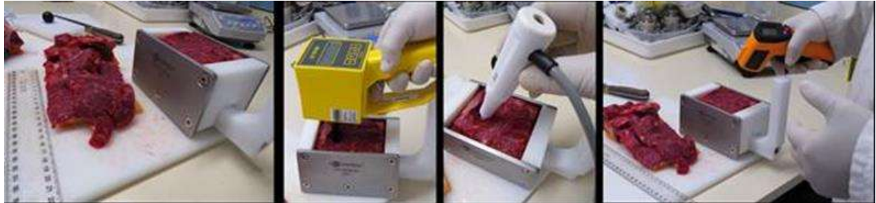
Figure 2. Preparation of meat blocks for treatment. The samples were cut to fit the PEF treatment chamber (dimensions of 13 × 8 × 5 cm) and the conductivity, pH and temperature were measured before and after treatment.
