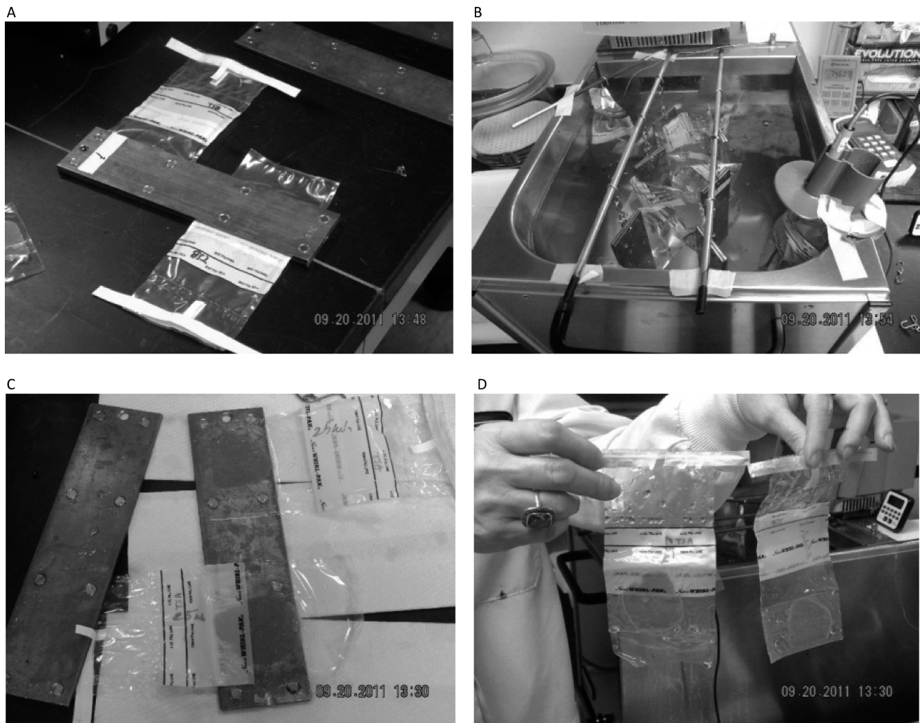
FIGURE 1. Setup of duplicate sample bags between magnetic copper plates before heating (A), immersion of samples in the heated water bath (B), and release of the samples after cooling (C) and (D).
