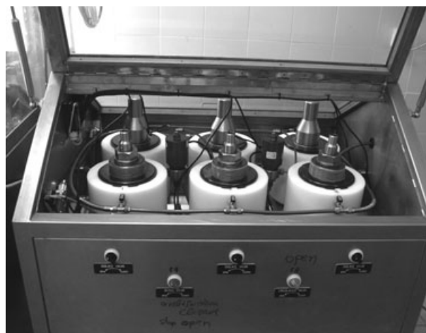
Figure 1 Block of six small (42 ml) high-pressure vessels (2.5 cm in diameter and 10 cm in length) used for the pressurization of the ham model system pouches.
