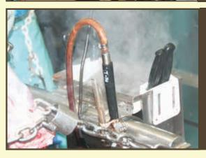
Dual knife system for sterilizing knives.
