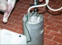
Lactic acid dispenser with gauges for monitoring temperature and pressure that, depending on the establishment's supporting documentation, may be critical operating parameters.
