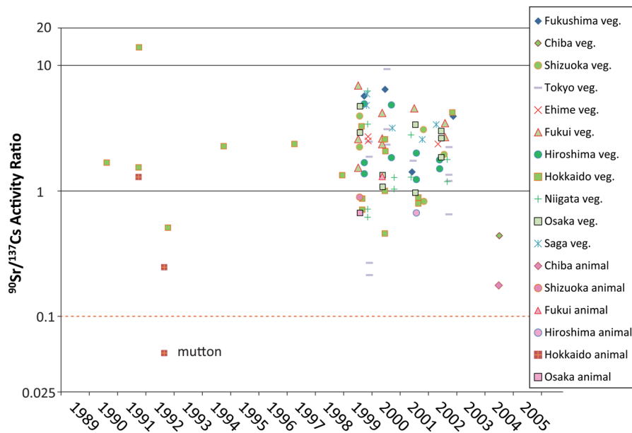
Figure 8. Activity ratios of ^{90}\text{Sr}/^{137}\text{Cs} in vegetarian produce and meat/egg products from Japan sampled and measured before the Fukushima nuclear accident. The dashed red line indicates the 10% limit that was assumed by Japanese authorities as the maximum ^{90}\text{Sr} content after the Fukushima accident.
