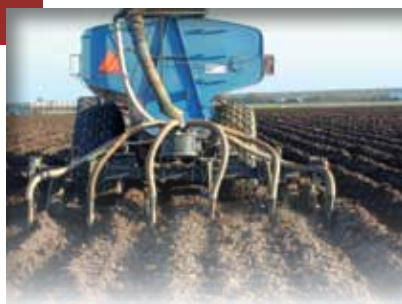
Liquid biosolids application via injection in Tucson, Arizona
