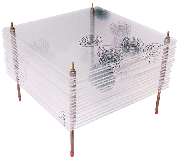
Three-dimensional map of part of one of the crystal salts of penicillin based on X-ray crystallography work by Dorothy Hodgkin and Barbara Low (Oxford) and C.W. Bunn and A. Turner-Jones (I.C.I. Alkali Division, Northwich). The work has been made available by the Museum of History of Science, University of Oxford under Wikimedia Commons for Ada Lovelace Day 2013 (source: © 2008 commons.wikimedia.org).
