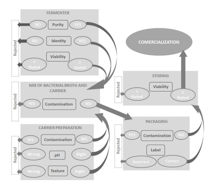
Figure 2. Quality control in the biofertilizer manufacturing process.
