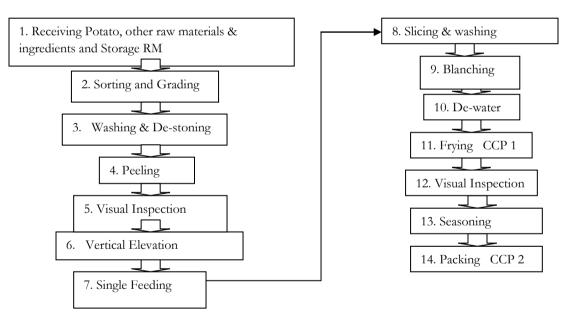
Figure-2: Process flow diagram of Potato Chips
