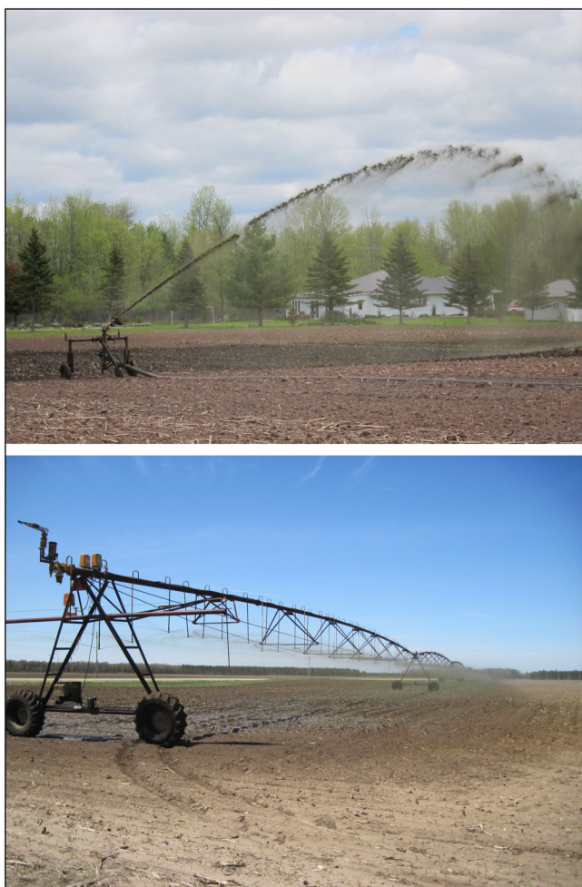
Figure 1. Photos of spray irrigation conducted using traveling gun (top) and center pivot (bottom) equipment. Photos taken by authors Mark Borchardt (traveling gun) and Rebecca Larson (center pivot).
