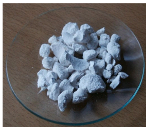
Fig. 8. Ash after the calcining of bone sludge at 950 °C.
