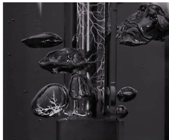
FIGURE 4 (a) Schematic diagram of the plasma-bubble generator. (b) Photograph of a discharge in a forming bubble. Reproduced from Mai-Prochnow et al. (2020) with the permission of John Wiley and Sons.
