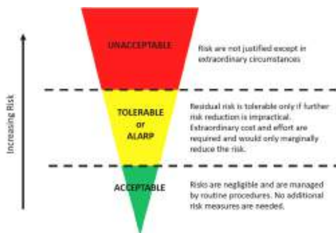
Fig. 4. Levels of risk under the “As Low as Reasonably Practicable” (ALARP) Triangle (Neilson et al., 2017).
